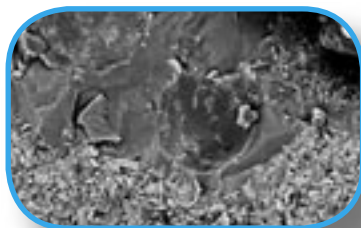
Oils and rocks. Chalk rock saturated with brine and oil. Dark grey bubbles are dried oil droplets in brine-filled cracks
