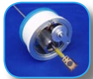
Cryo transfer device with specimen shuttle and stub insert
