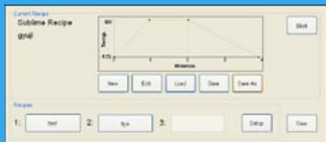
Sublimation parameters for temperature and time can be pre-set and stored
