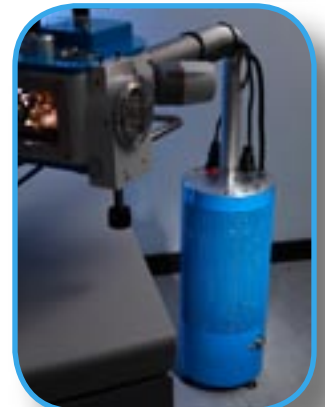
Off-column turbo-pumping system
